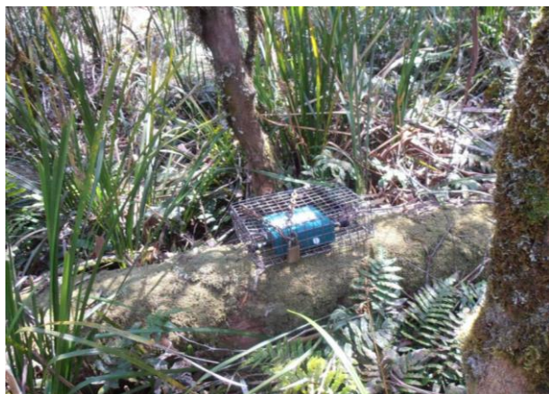
Figure 1. The Song Meter™ installed at the Munro Hut Rufous Scrub-bird territory.
